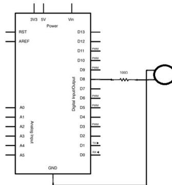
**Fig. 2.** Connection of piezoelectric element with microcontroller
