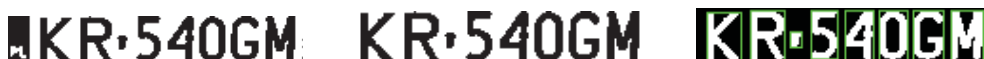
Figure 23. Character segmentation stages: left: horizontal region of interest selected, center: vertical region of interest selected, right: separated characters.
