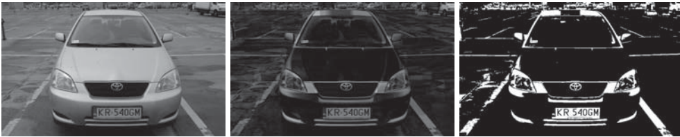
Figure 20. Initial preprocessing of the algorithm: left: conversion to gray scale, center: after a white top hat operation, right: black and white thresholded image.
