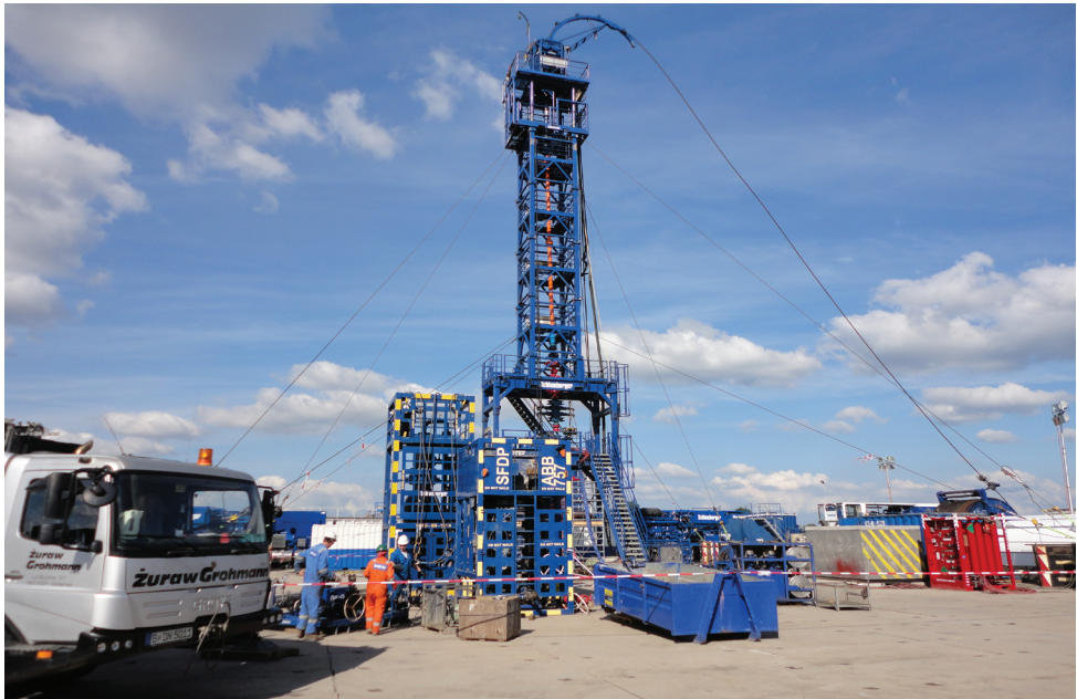
Fig. 4. Frac head including BOP'S and coiled tubing [4]
