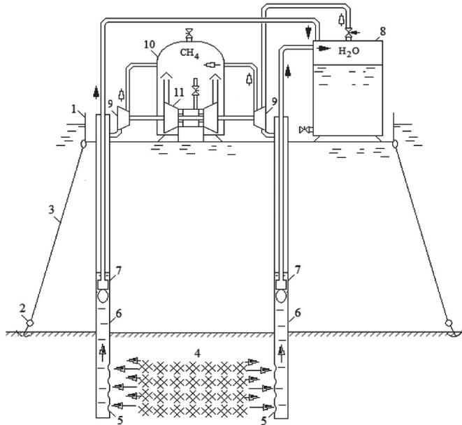
**Fig. 2.** Schematic diagram of the plant for the extraction of methane gas and fresh water from the gas-hydrate deposit by lowering the pressure (decompression). 1 – a platform for placing equipment of the installation; 2 – anchor; 3 – ropes; 4 – gas-hydrate layer; 5 – windows for the removal of the gas-water suspension from the formation into the pumping well; 6 – pumping well; 7 – submersible electric pump; 8 – fresh water tank; 9 – the compressor; 10 – gasholder; 11 – gas turbine drive
