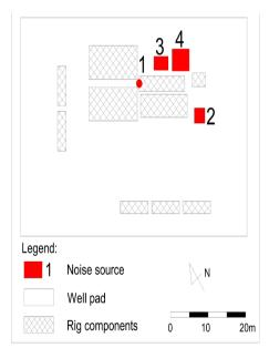
Fig. 3. Major sources of noise during the realization of the gas well Wieczorek-AGH-1 (1 – driving head, 2 – mud pump EMSCO HTF 500, 3 – air compressor Atlas Copco XRVS336, 4 – air compressor Atlas Copco XRXO667)
