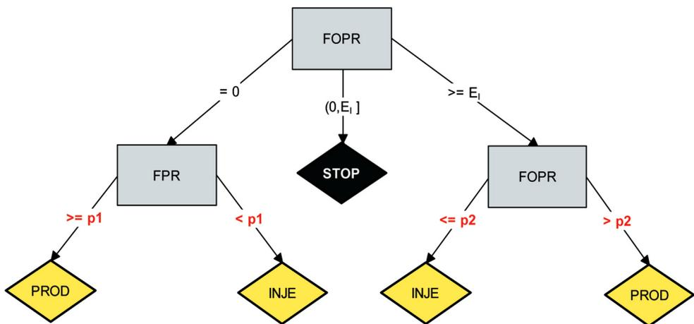
**Fig. 1.** Parameterized decision tree developed for the CO<sub>2</sub>-EOR process
