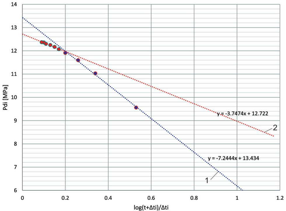
**Fig. 2.** Determination of linear regression equations for two sections of the bottom pressure build-up curve recorded in the first cycle of the DST test in the W-3 well
