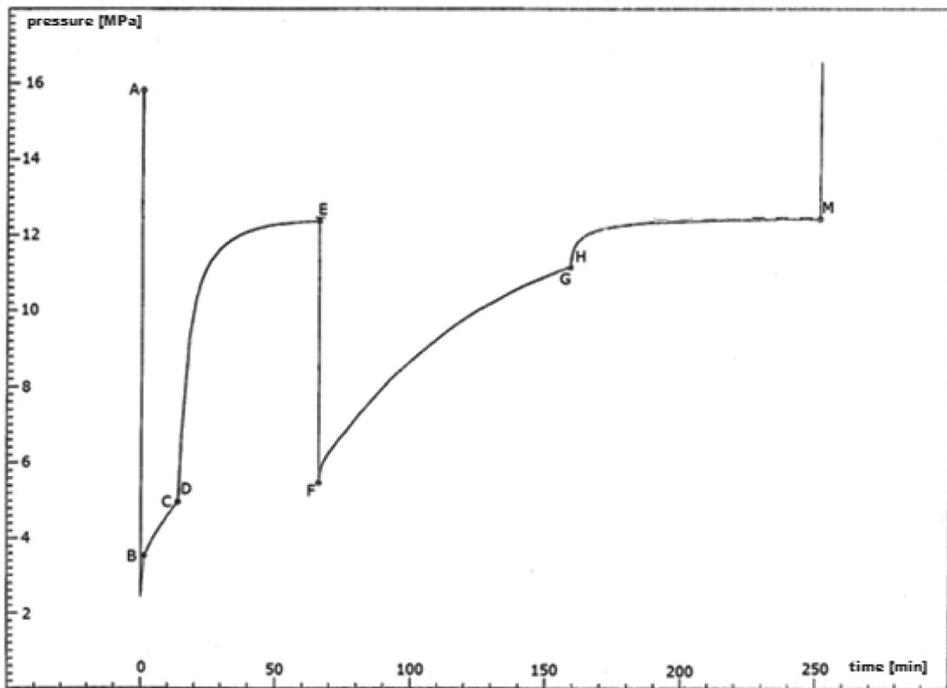
**Fig. 1.** Diagram of changes in bottom pressure recorded during a two-cycle DST test of Mesozoic strata in the W-3 well [4]
