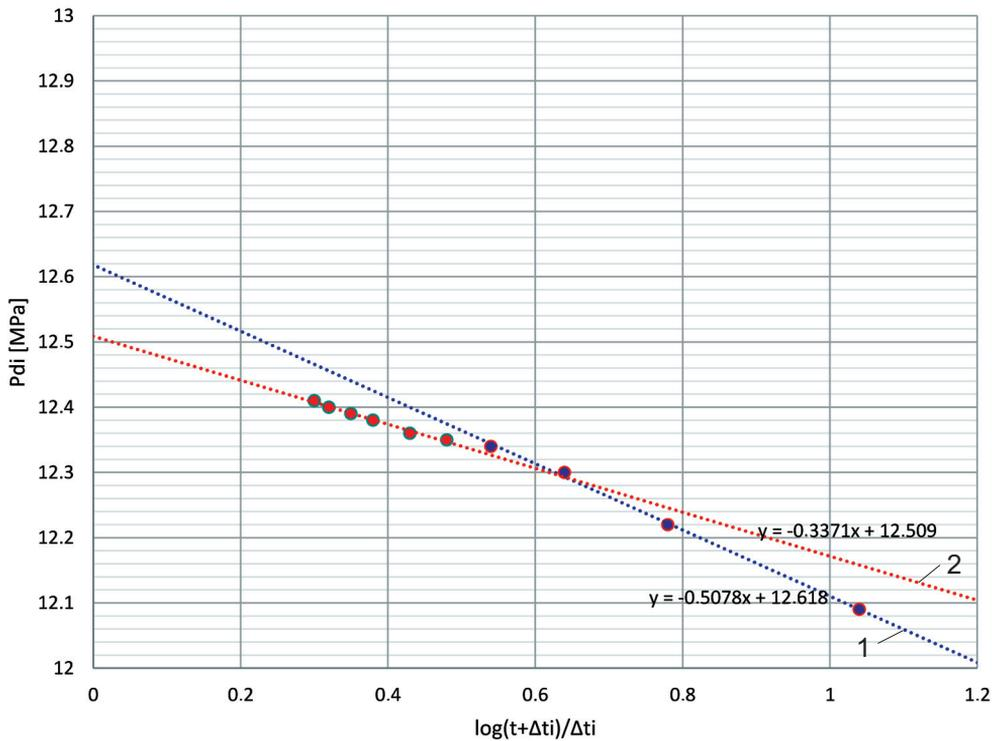
**Fig. 3.** Determination of linear regression equations for two sections of the bottom pressure build-up curve recorded in the second cycle of the DST test in the W-3 well
