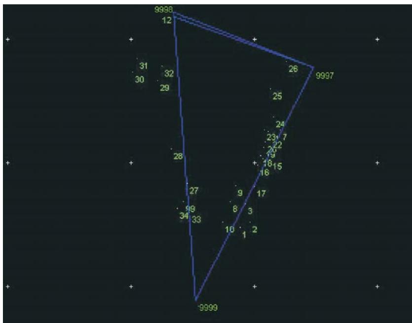
**Fig. 1.** The draft of traverse with points measured in positional and altitude way – the Geonet program
