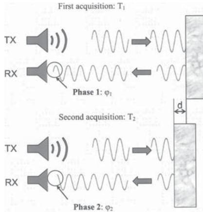
Fig. 3. Phase shift as a result of displacement of the object
