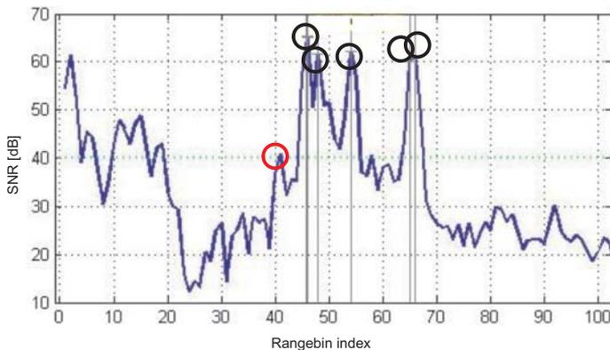
Fig. 13. Radar profile of the surveyed footbridge
