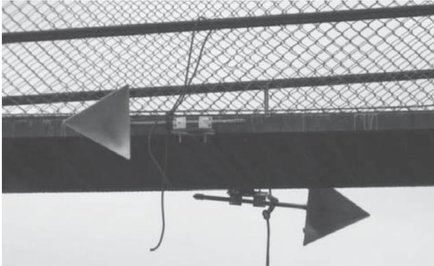
**Fig. 2.** Horn reflectors installed on the object
