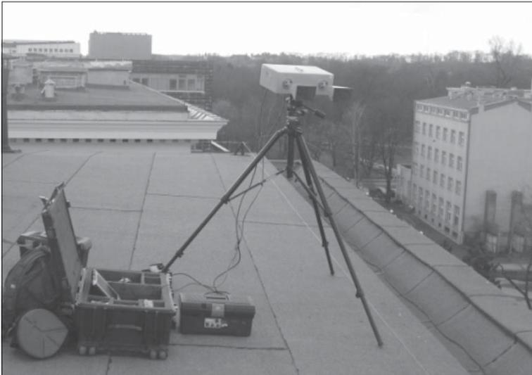
Fig. 1. IBIS-S system during the surveys
