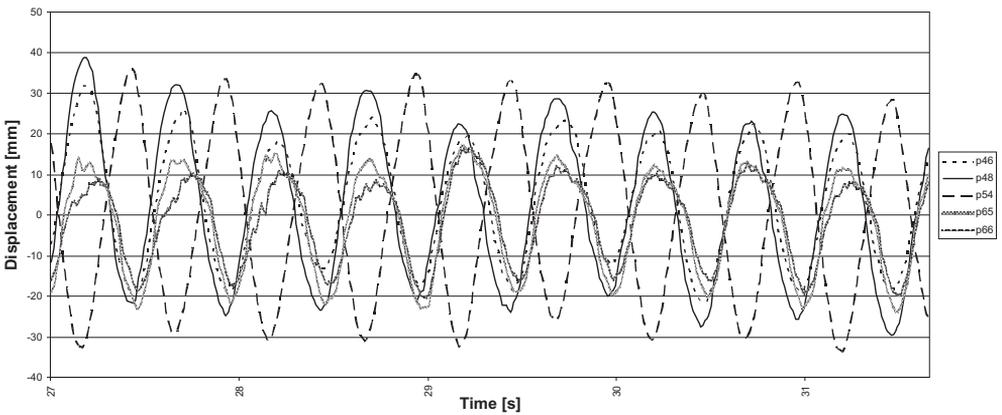
Fig. 8. Contrary vibrations of the footbridge mid-point in relation to the others
