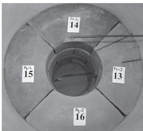
**Fig. 3.** Position of segments in the experimental vessel
