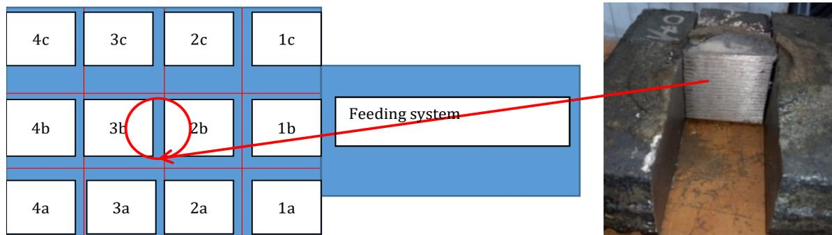
Fig. 4. Ingot cutting for analysis
