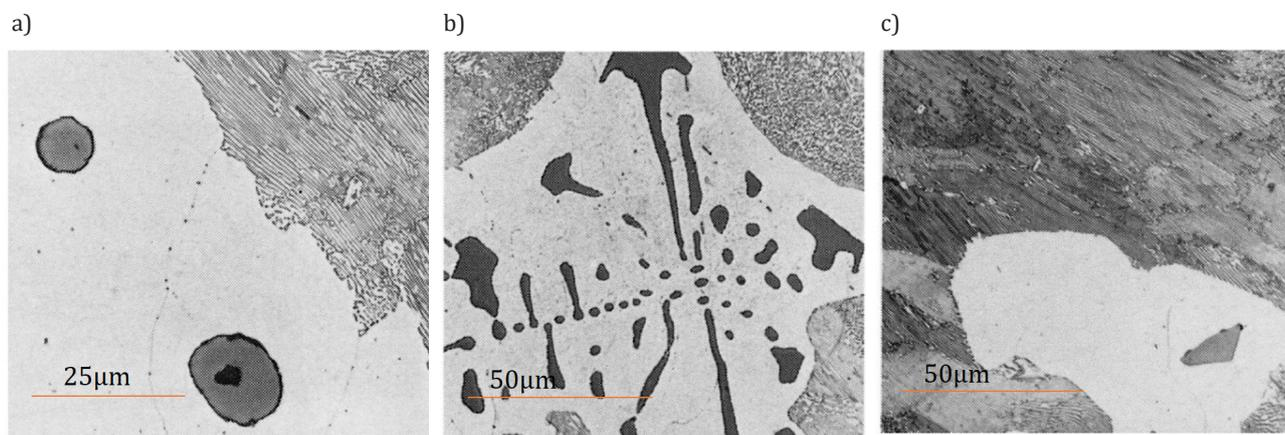
Fig. 1. Example of sulfur inclusion: a) Type I,  $\times 800$ ; b) Type II,  $\times 500$ ; c) Type III,  $\times 500$  [9]
