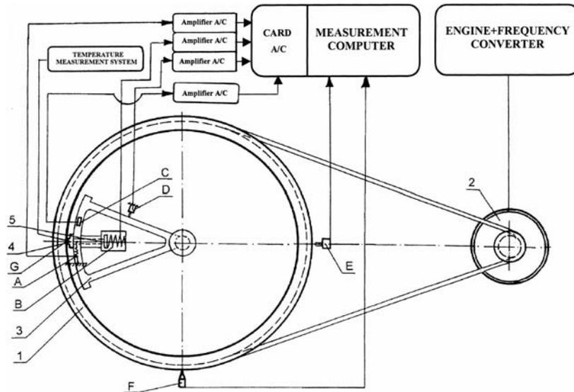
Fig. 2. Scheme of testing stand measurement system
