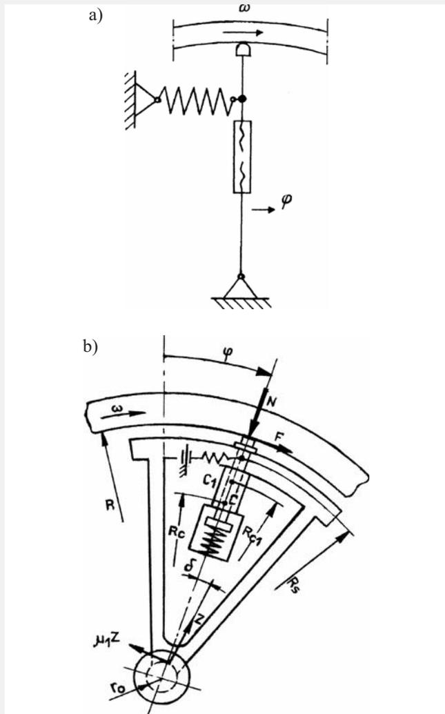
Fig. 1. Scheme (a) and construction (b) of testing system
