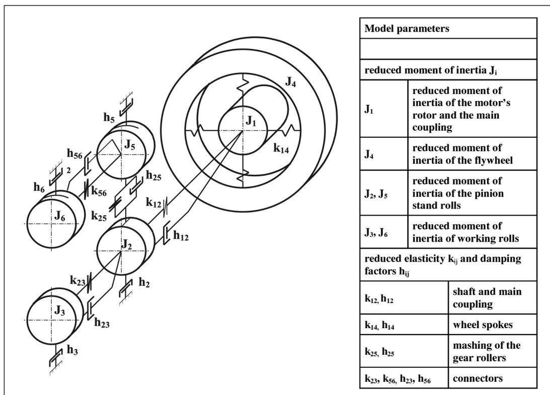
Fig. 6. Mass spring model of a pilger mill's drive reduced to a 6-DOF system
