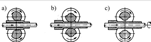
Fig. 1. Operating principle of a pilger mill (schematic diagram)
