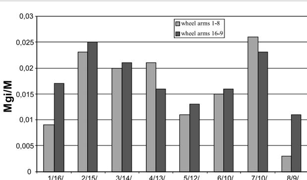
**Fig. 4.** Contributions of individual wheel arms to the transmission of inertia force moment. Condition after one year of service
