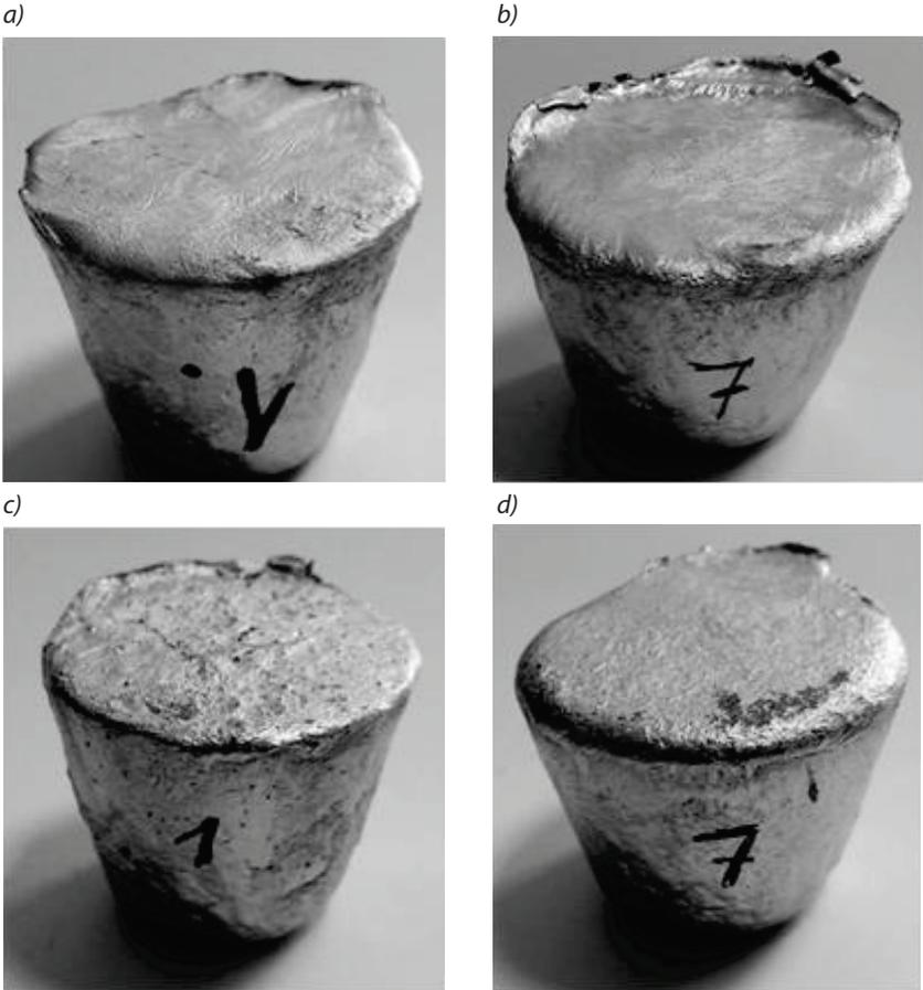
Fig. 5. Samples selected from individual melts solidifying under decreased pressure: induction thiristor furnace (samples a and b); silite furnace (samples c and d)
