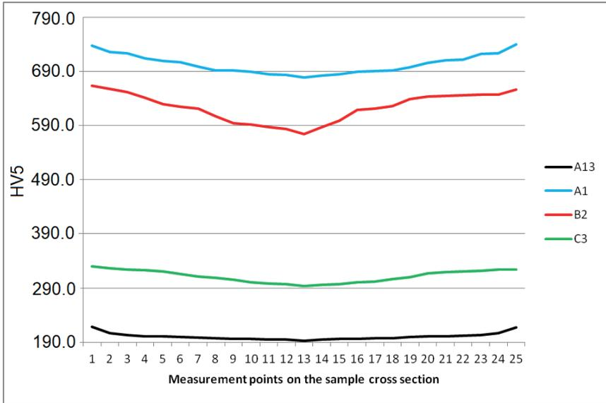
Fig. 4. Graphs of ball hardness obtained from 100Cr6 steel rolled in the conventional method, cooled in three quenching media
