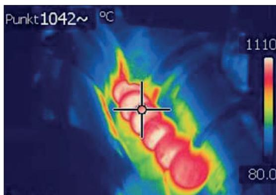
Fig. 1. Temperature measurement of rolled balls in skew rolling mill, view from the output
