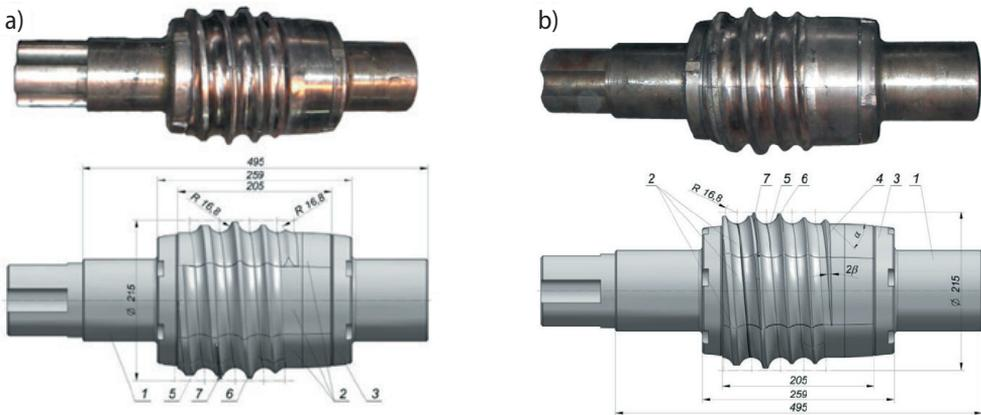
Fig. 2. Sets of screw segments tools for rolling the balls: a) conventional method; b) modified method; description in the text
