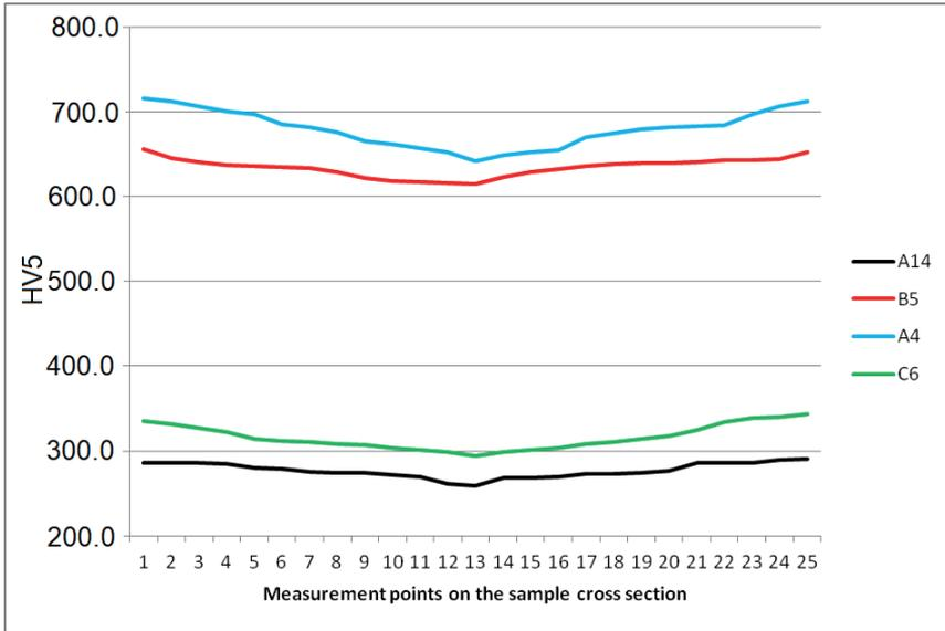
Fig. 6. Graphs of ball hardness obtained from steel cut from railway rail rolled in the conventional method, cooled in three quenching media
