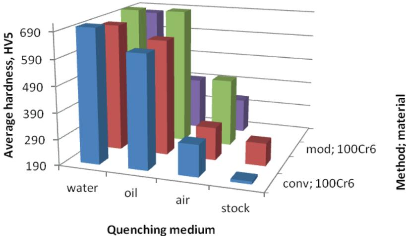
Fig. 8. The mean hardness of the analyzed samples
