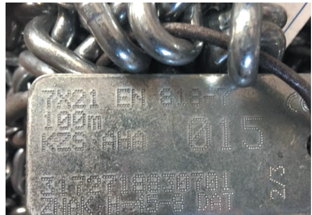
Fig. 4. Mark placed every meter at the ends of a chain
