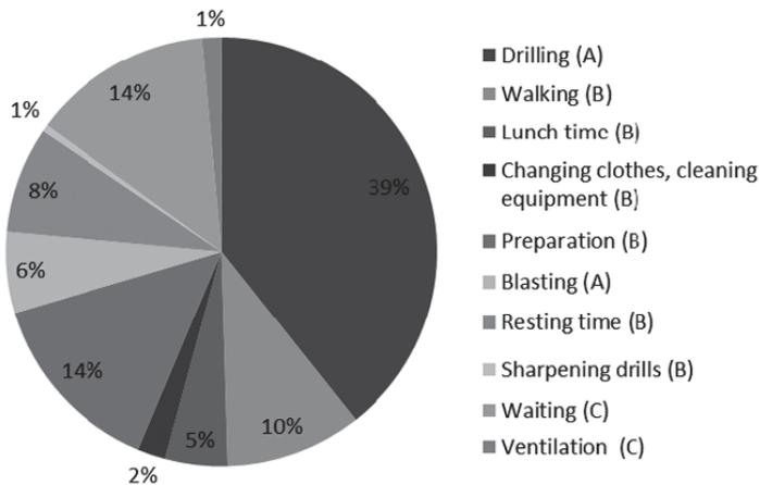
Fig. 1. Operations carried out in a mining block
