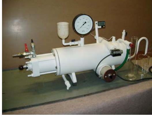
Fig. 1. The measuring instrument of MAF VII series with the pressurising piston (model 2005)
