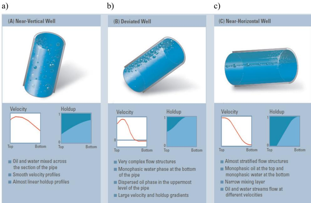
**Fig. 2.** Three main types of flow structure can occur in a two-phase (water-oil) system: a) near-vertical well; b) deviated well; c) near-horizontal well
