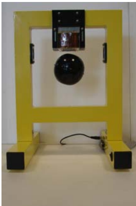
Fig. 1. Photo of the laboratory AMLS (a). Diagram of the AMLS with one electromagnet (b) [8]
