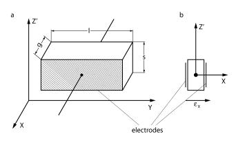
Figure 2. Optical axis of quartz plates used in phase I experiments. a - Z', Y, X - optical axes, s, l, b - parameters of plate, $\epsilon_1$  – frequency of plate vibration (which is a function of the thickness of plate)
