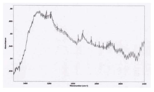
**Figure 4.** IR curves of aspartic acid on quartz plates. The lower curve is still (not vibrating), the upper is vibrating, at a frequency of 8580 kHz. The position of the absorption peak changes during vibration
