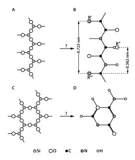
Figure 1. Similarity of selected mineral and organic structures A – the structure of chain silicate (Bolewski 1965), B – structure of peptide chain (Lasek 1978), C – structure of layered silicate (Bolewski 1965), D – structure of cytozine, one of most important DNA component (Jerzmanowski 1994)
