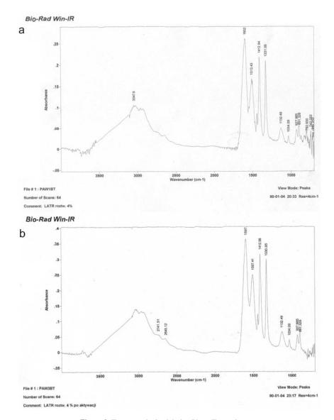
**Figure 9.** IR curves obtained during Phase II experiments. a – glycine dissolved in water (stable conditions), b – glycine at vibrating conditions (quartz mixed with dissolved glycine treated by artificial lightning)
