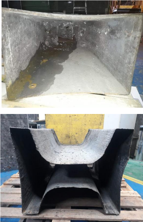
Fig. 2: Solid shell off a bloom and beam blank
