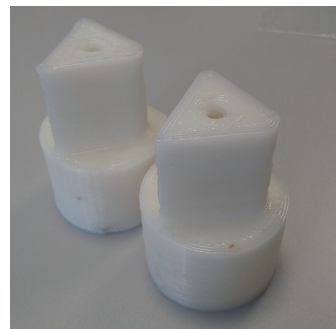
Fig. 5. Final pieces with residual pressure compensation
