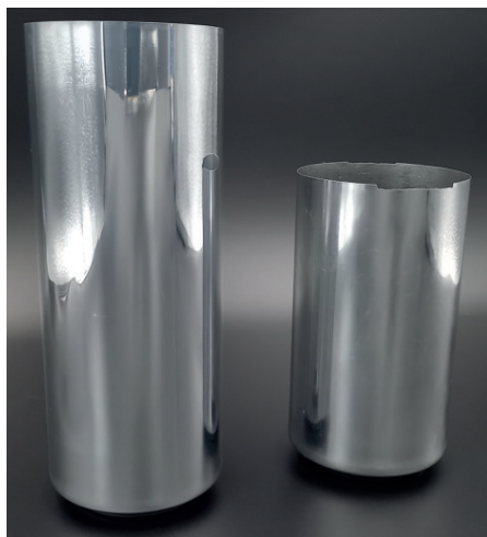
Fig. 1. Normal can (left) and the analysed defect – a “short can” (right)
