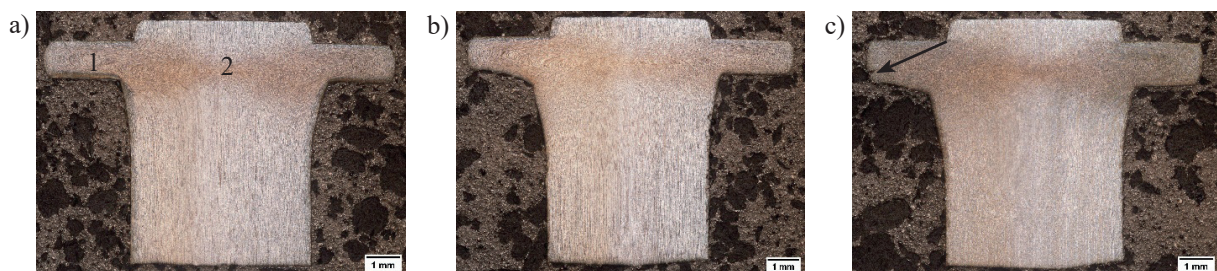
Fig. 6. Macrostructure of the cold-headed samples of wire rod of 32CrB4 steel after the following variants of cooling: a) variant W280; b) variant W395; c) variant W440. The average strain rate was 10 \text{ s}^{-1}
