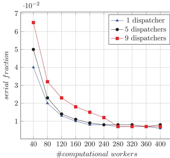
**Figure 6.** Serial fraction as a function of the number of computational workers for one, five and nine computational task dispatchers.
