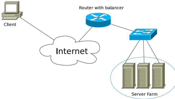
**Figure 2.** Router load balancing.
