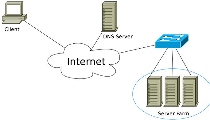
**Figure 1.** DNS load balancing.
