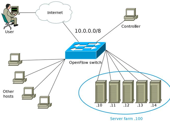
**Figure 6.** System architecture.
