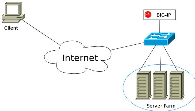
**Figure 3.** F5 load balancing.
