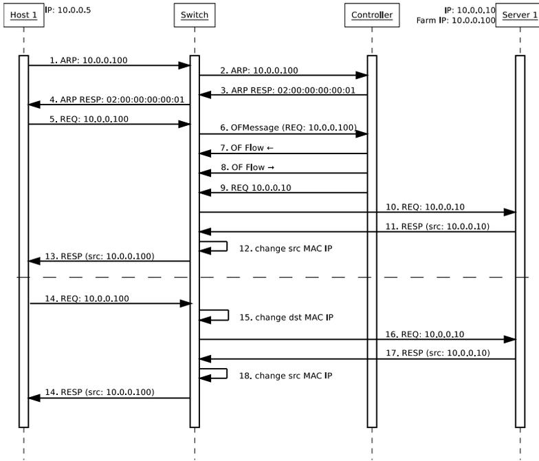
**Figure 8.** Detailed request path through the network.
