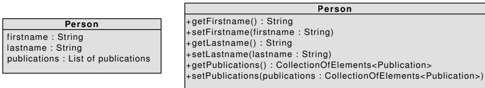
Figure 5. Correspondence between a logical type (on the left) and its Java implementation (on the right). Parameters are simply converted into setter-getter pairs. Lists of elements are implemented as special collections.
