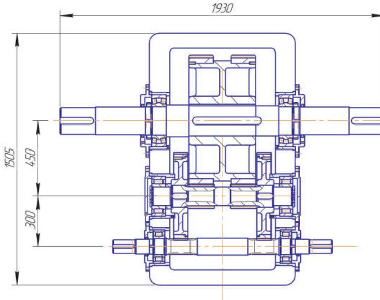
**Fig. 1.** Reducer TS2NSH-750 of pumping unit
