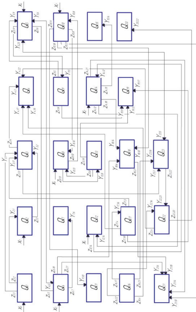
**Fig. 4.** The logical diagnostic model of the pumping unit reducer
