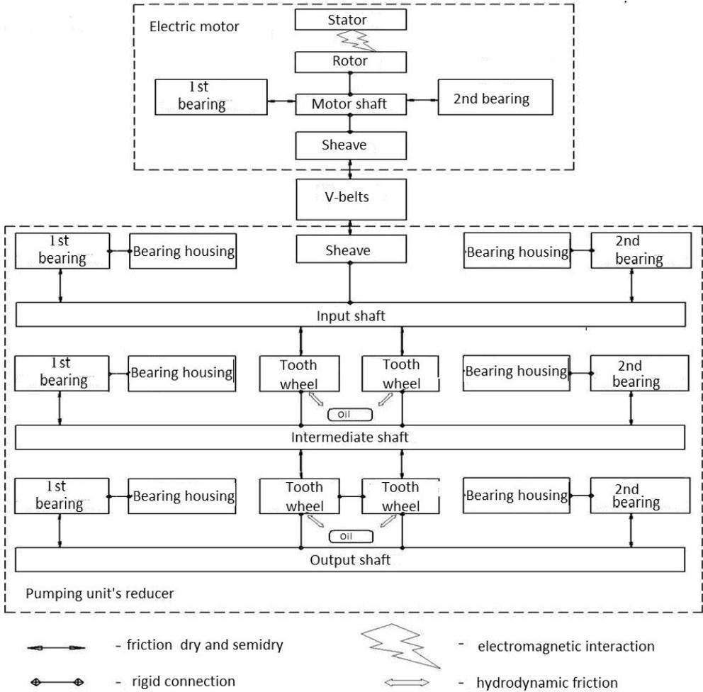
Fig. 2. Functional diagram of the pumping unit reducer
