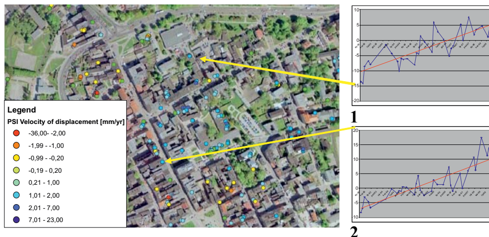
Fig. 2. Distribution of PS points in the Inowrocław Old Town area; uplifting trend with the average elevation of 3 mm/year
