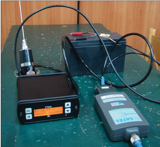
Fig. 3. IGTS-R with a connected radio modem during the tests
