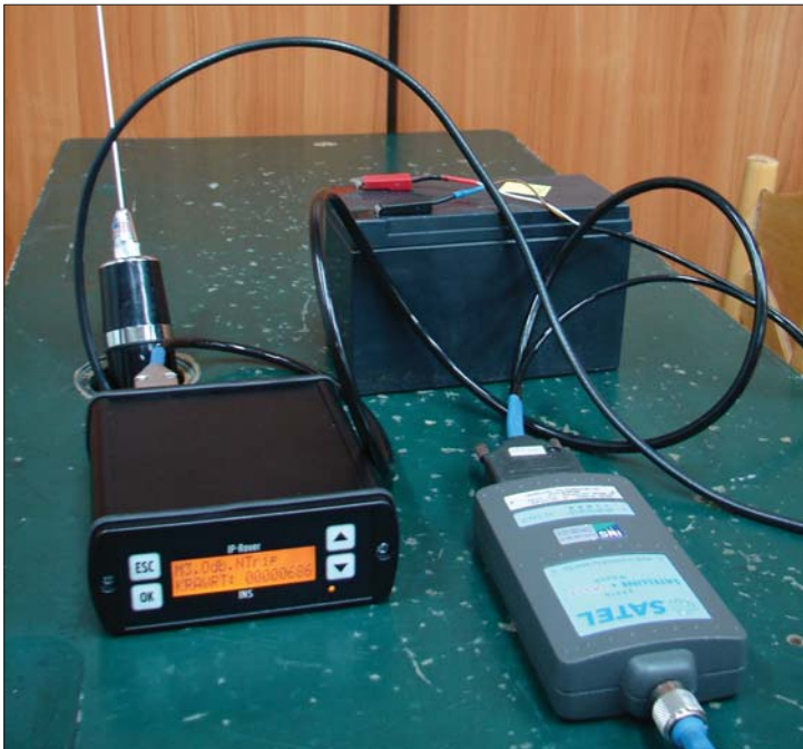
Fig. 6. Base station emulation by an IGTS + radio modem configuration
