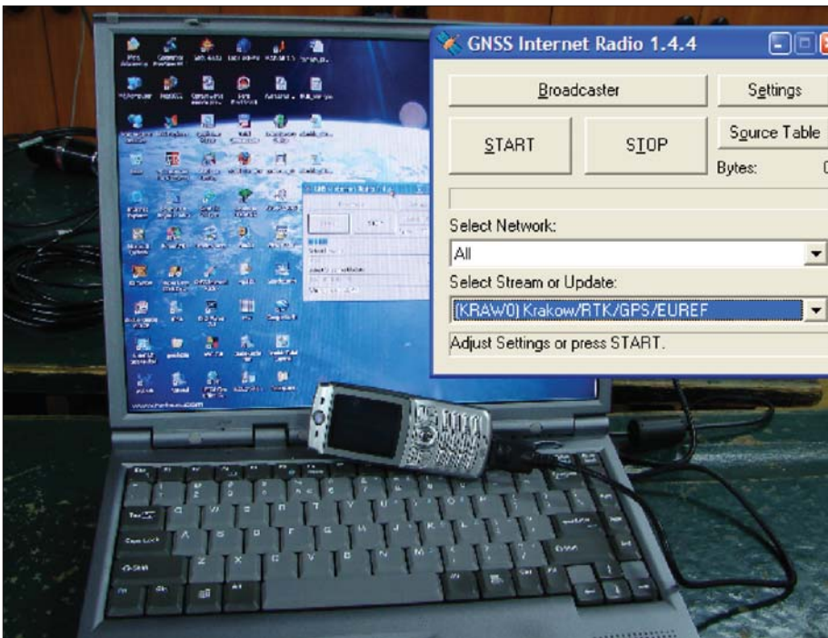
Fig. 4. Program GNSS Internet Radio on a computer connected to Internet via GPRS using a mobile phone
