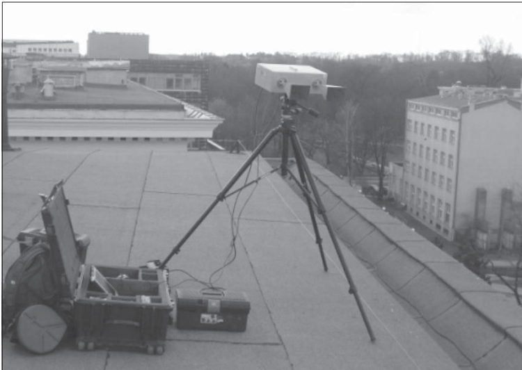
Fig. 1. IBIS-S system during the surveys
