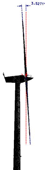
Fig. 9. Inclination angle of blade rotation planes relative to vertical line during operation
