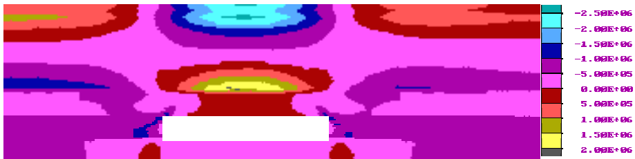
Fig. 1. Stress distribution in the first breakage of the key stratum with the mining height of 4 m
