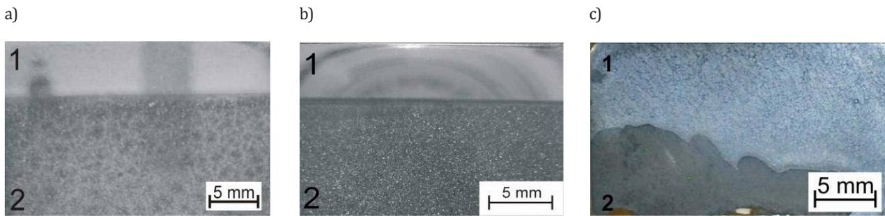
**Fig. 3.** Views of sample cross-section of layered castings in configuration: a) 1 – working layer in the form of a stainless steel X6Cr 13 grade plate, 2 – base part of grey cast iron; b) 1 – working layer in the form of a stainless steel X2CrNi 18-9 grade plate, 2 – base part of grey cast iron; c) 1 – base part of carbon cast steel, 2 – working part in the form of Cr-base layer
