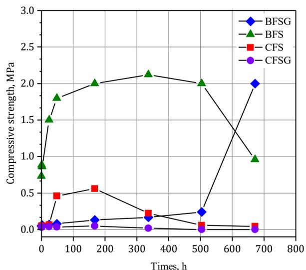
Fig. 2. Measured values of compressive strength of metallurgical slags after different times of hardening
