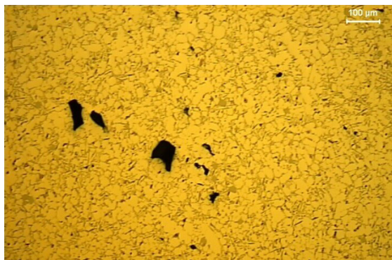
Fig. 4. Microstructure of casting made of alloy with initial Mn content (0.29%)
