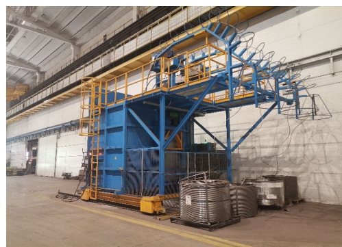
Fig. 4. The station for spheroidization and modification with the PE method
