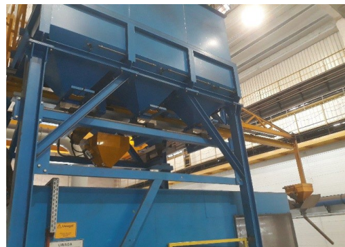
Fig. 3. Automated system for introducing modifiers on the metal stream when pouring into a ladle
