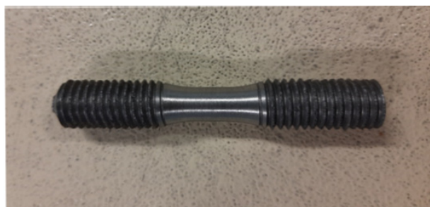
Fig. 3. Gray iron tensile strength sample made according to the customer's standard. Diameter of the sample D = 6 mm, length without fixings L = 15 mm
