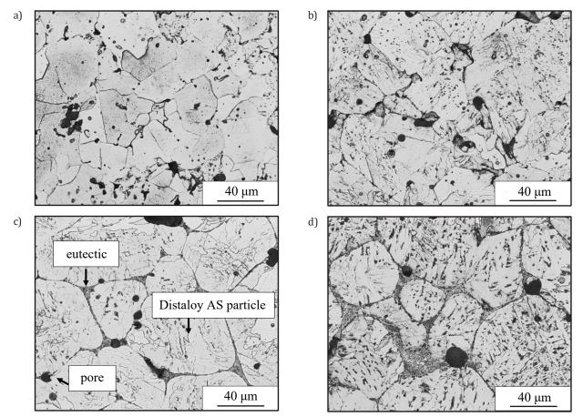
Fig. 5. Microstructure of Distaloy SA sinters alloyed by boron for 70–100 µm particle fraction: a) 0.0 wt.% B; b) 0.2 wt.% B; c) 0.4 wt.% B; d) 0.6 wt.% B
