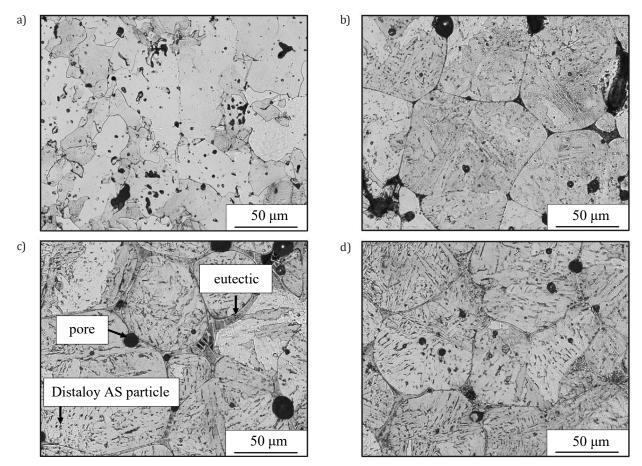
Fig. 6. Microstructure of Distaloy SA sinters alloyed by boron for 40–56 µm particle fraction: a) 0.0 wt.% B; b) 0.2 wt.% B; c) 0.4 wt.% B; d) 0.6 wt.% B
