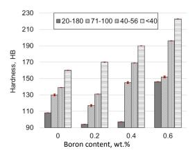
Fig. 3. Effect of powder particle fractions and boron contents upon the hardness of prepared sinters: fraction 20–180  $\mu$ m, 71–100  $\mu$ m, 40–56  $\mu$ m, and < 40  $\mu$ m
