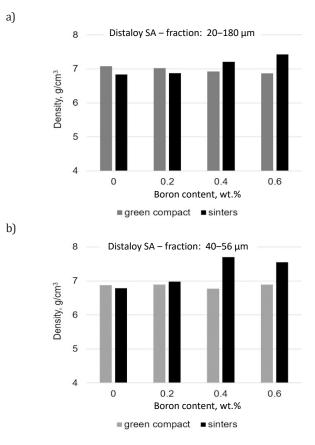
Fig. 1. Effect of particle fraction of powder and boron addition upon density of green compacts and sinters: a) 20–180  $\mu m$  fraction; b) 40–56  $\mu m$  fraction
