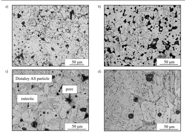
Fig. 7. Microstructure of Distaloy SA sinters alloyed by boron for <40 µm particle fraction: a) 0 wt.% B; b) 0.2 wt.% B; c) 0.4 wt.% B; d) 0.6 wt.% B
