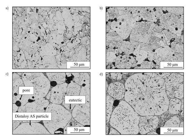
Fig. 4. Microstructure of Distaloy SA sinters alloyed by boron for 20–180 µm particle fraction: a) 0.0 wt% B; b) 0.2 wt% B; c) 0.4 wt% B; d) 0.6 wt% B [7]
