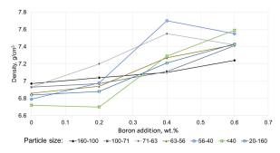
**Fig. 2.** Density of Distaloy SA sinters for all used powder fractions with boron addition in respect to particle fraction of powder
