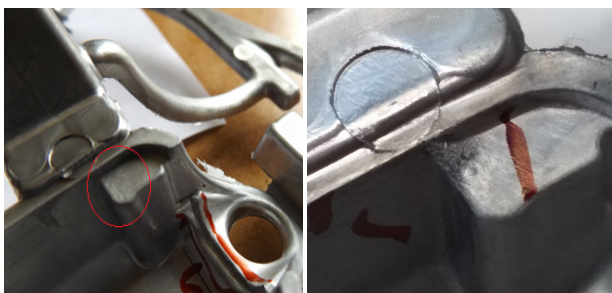
Fig. 5. Areas of remaining castings visually inspected at beginning of mould life and 30% of mould life
