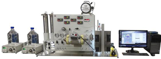
Fig. 1. Bench-top relative permeability system
