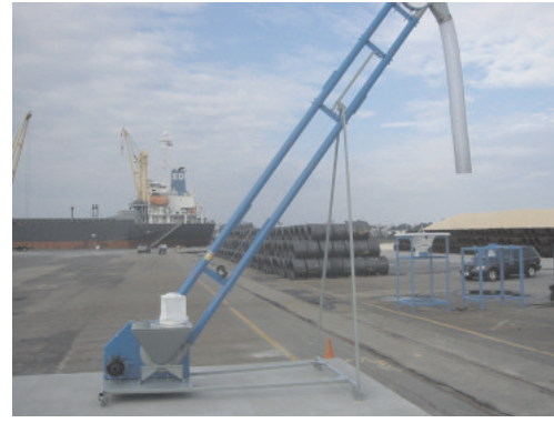
Fig. 1. Example of application of scraper pipe conveyors for loading vehicles and railway carriages (Krause et al. 1999)
