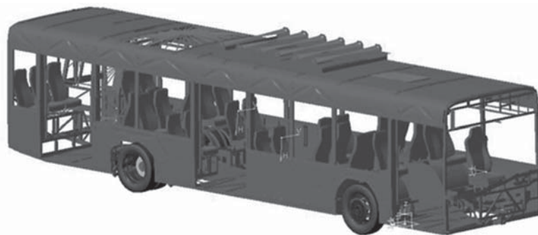
Fig. 4. Coupled rigid- flexible multibody model
