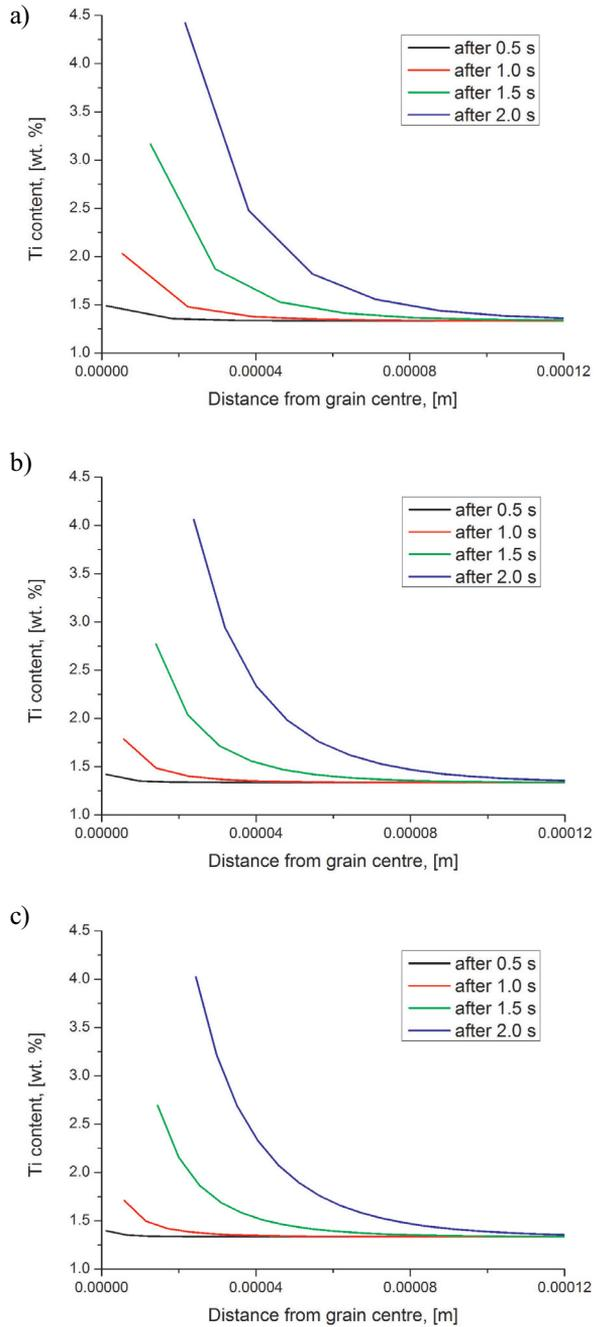
**Fig. 1.** Ti concentration in liquid adjacent to the dendrite tip after 0.5, 1, 1.5, 2 seconds since grain initiation. Results of computations for grids of different density: a) 30 points; b) 60 points; c) 90 points
