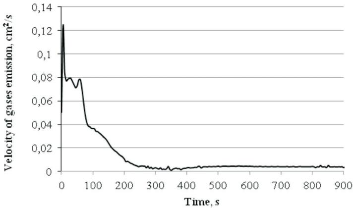
**Fig. 5.** Kinetics of gas emission from BioCo2 bonded moulding sand
