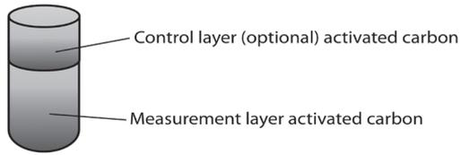
**Fig. 2.** Scheme of container with the activated carbon
