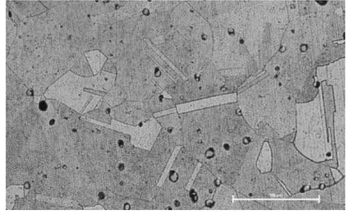
**Fig. 2.** Copper bracelets, Clo (Site 7), 3500 BC. Microstructure of the copper artefact, with discernible precipitates of  $\text{Cu}_2\text{O}$  oxygen phases against the background of grains of the copper matrix; magnification: 100x (a) and 500x (b)
