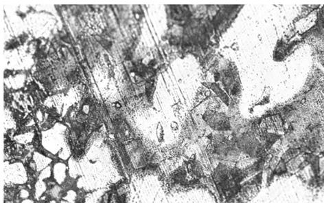
**Fig. 6.** Bronze torque, Krzesławice (Site 41), 1<sup>st</sup> century BC. Microstructure of the tin-lead bronze cast, with discernible dendritic segregation of tin and lead in the spaces between crystallites of the  $\alpha$  solution; magnification: 200x (a) and 500x (b)
