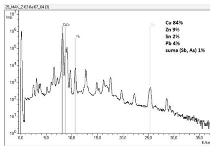
**Fig. 7.** Bronze buckle, Zesławice (Site 63), 600 AD. a) the view, b) the X-ray spectrum with identification lines for copper, zinc, tin and lead. Concentration of elements: copper – 84%, zinc – 9%; tin – 2%; lead – 4%; other admixtures – 1%
