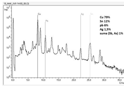
Fig. 5. Bronze torque, Krzeslawice (Site 41), 1<sup>st</sup> century BC: a) the view, b) the X-ray spectrum with identification lines for copper, tin, lead and silver. Concentration of elements: copper – 79%; tin – 12%; lead – 6%; silver – 1.5%, other admixtures – 1%
