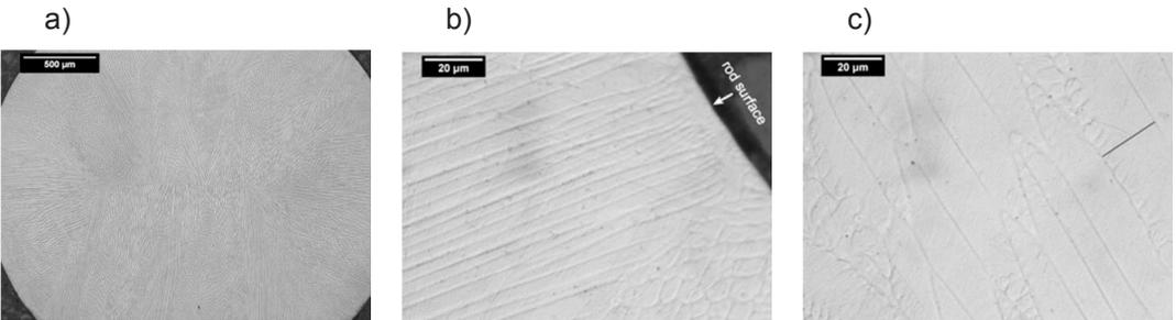
**Fig. 2.** Microstructures of the suction-cast Fe-25Ni alloy: a) cross-sectional image of the rod cut in half crosswise (light microscopy, 50x), b) magnified area close to the rod surface and c) in the rod axis (light microscopy, 1000x)
