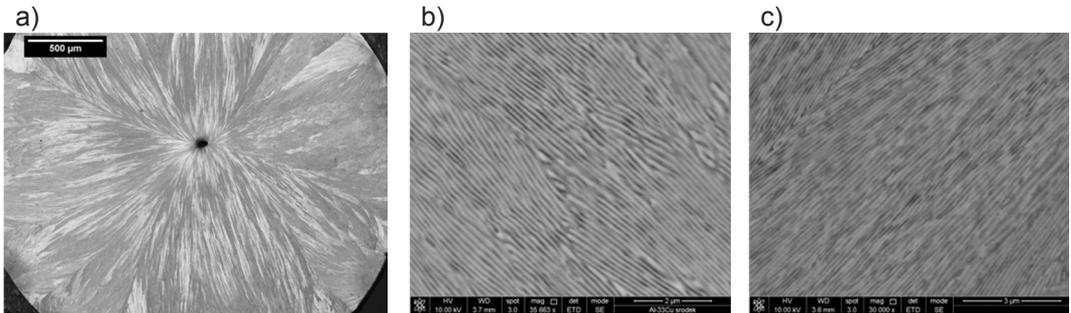
**Fig. 5.** Microstructures of the suction-cast Al-33Cu alloy: a) cross-sectional image of the rod cut in half crosswise (light microscopy, 50x), b) magnified area close to the rod surface and c) in the rod axis (scanning electron microscopy, 30000x)
