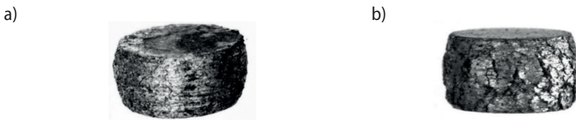
Fig. 7. Images of the samples after compression test for the addition of 10 wt% of SiC with particle sizes of: a) 2 \mu\text{m} ; b) 40–60 \mu\text{m}
